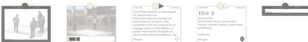
Figure 54: Active areas on the container; drag/selection rim, video buttons, toggle local content, scroll text, and drag/selection rim.
